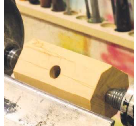
▲ Pic.21 Cutting the corners off the blank makes roughing out easier. By drilling the 13mm hole first there will be no chance of the hole breaking out, like there could be if drilled when the piece was round
